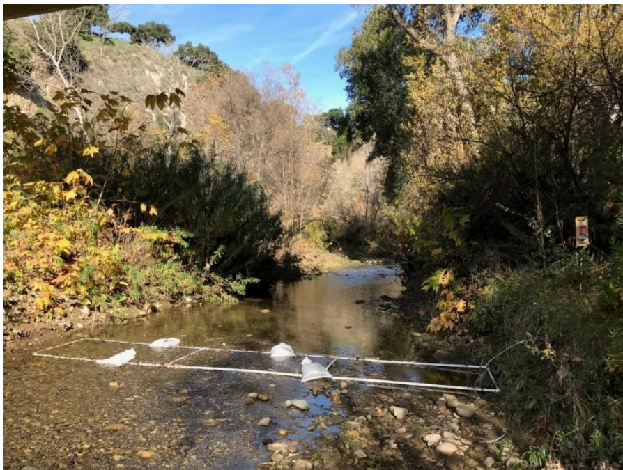
Figure 3: San Antonio Creek PIT tag array. The top image shows the solar panel and topside reader box. The lower image (facing upstream) shows the antenna in the stream and the tuner box mounted on a post on river left.
