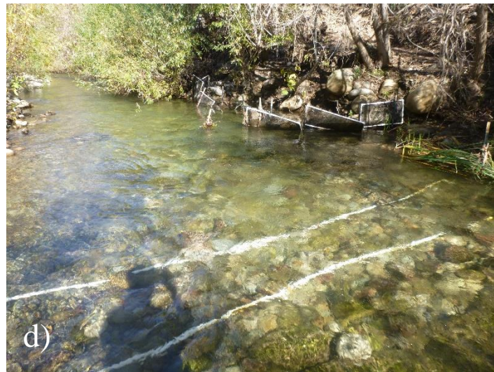
Figure 2: Ventura DIDSON and PIT tag array site. a) DIDSON and ARIS parallel configuration on river left with paneling upstream and downstream of cameras. b) View from stream bank showing the tuner box mounted to a large metal pole and the antenna on the streambed. c) View of the DIDSON and ARIS cameras during a high flow and turbidity event. d) View looking upstream at the PIT Tag antenna and DIDSON and ARIS cameras
